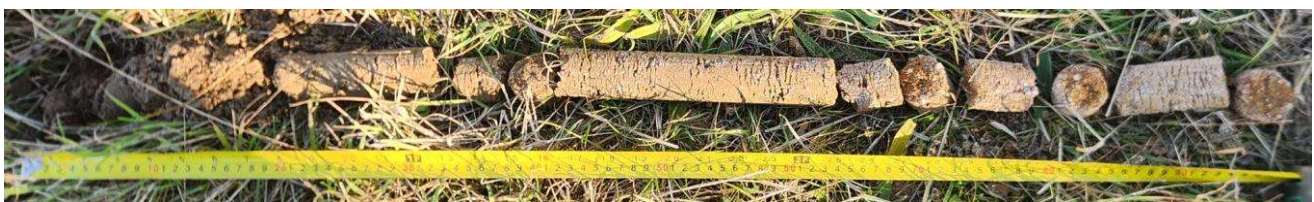
Figure 3.1: Borehole 3 – Typical soil profile
